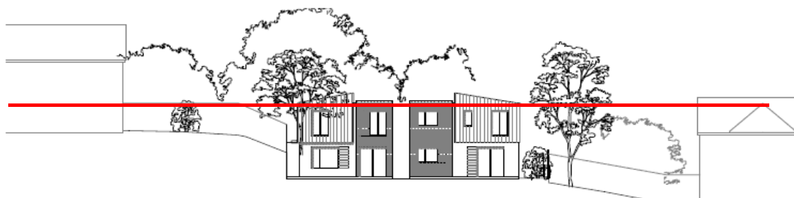
Figure 2. Section plan showing height of buildings in comparison to dwellings in Hollycroft Close and Ward Close
